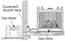
Figure 23 - Checking Gas Joints for Natural Gas Fireplace
